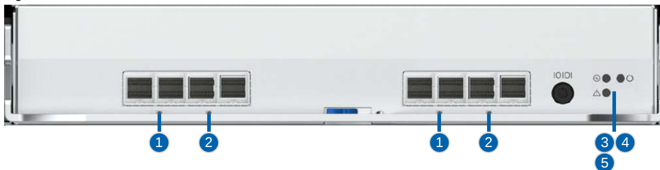
Figure 4-13 I/O module LEDs of JBOF
