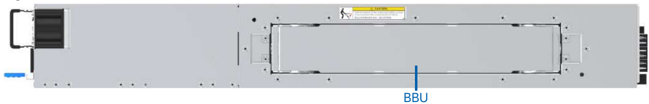
Figure 2-9 BBU module of control enclosure
