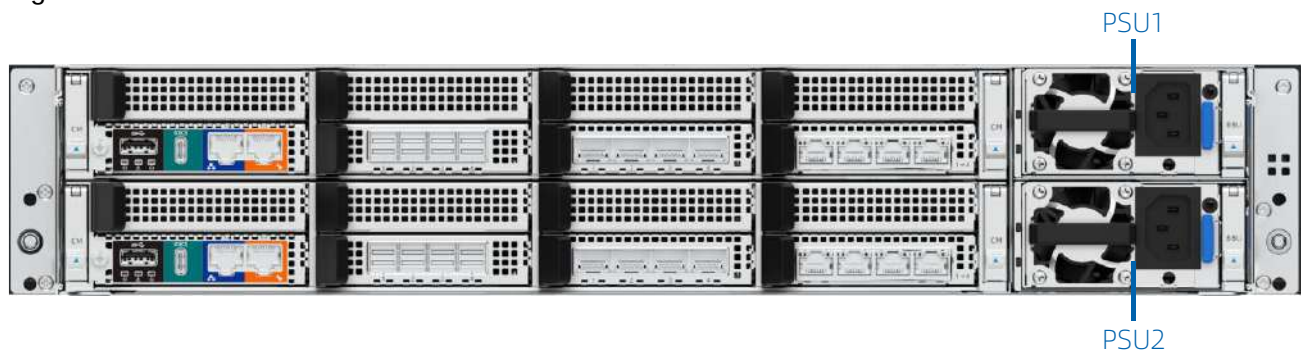
Figure 2-8 PSU modules of control enclosure
