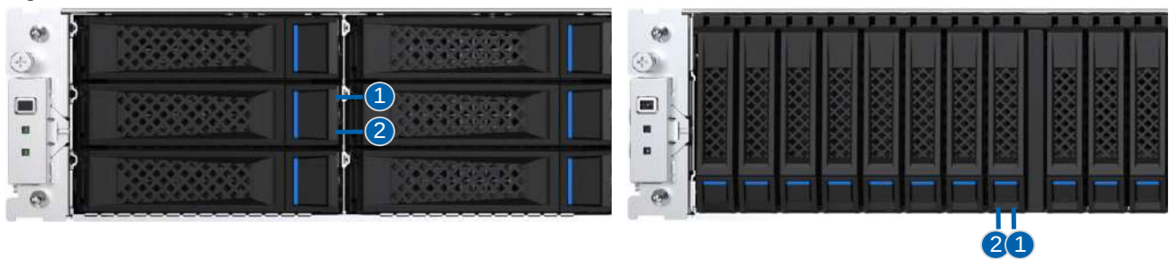
Figure 4-7 Disk LEDs of 2U JBOD
