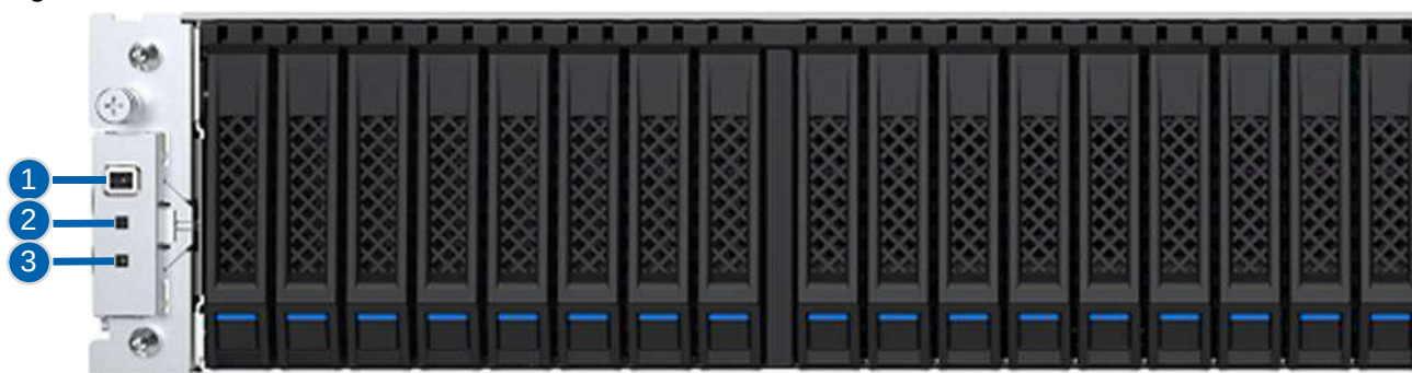
Figure 4-5 Enclosure LEDs of JBOD
