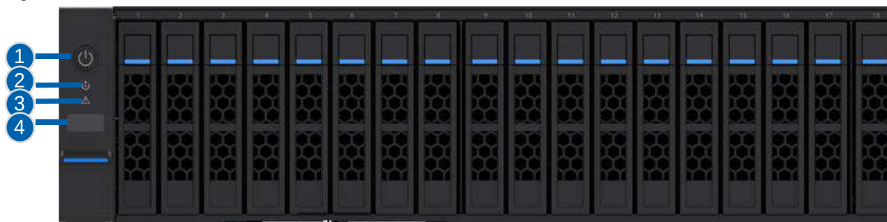
Figure 4-1 Enclosure LEDs of control enclosure
